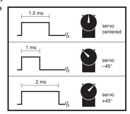
(R)ange, a position value of 0 corresponds to 0.5-ms pulse; 254 to 2.53 ms. A 1-unit change in position value produces a 8-microsecond change in pulse width. Positioning resolution is 0.72 degrees/unit (180 degrees/250).
