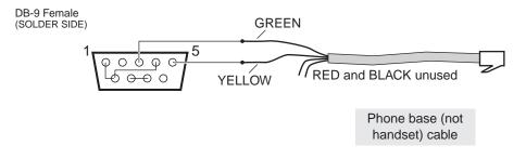
The connections between pins (1-9-4 and 7-8) are needed only if the programming language you're using can't turn off serial port handshaking. QBASIC, the language used in the PC example program, doesn't require these connections.
